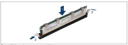
Figure 33: Inserting a memory module
